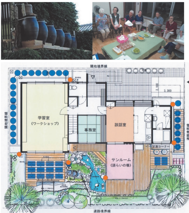
Fig.10 Implementation example at existing detached house (Barrels/Pond/Rainwater footbath/Infiltration to the soil/Gardening)
