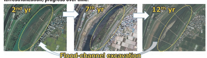
Fig. 5. Conceptual diagram of cyclic floodplain rejuvenation using flood channel excavation in a specific site in a target river segment. Time elapsed following excavation is shown in each photograph. Tree establishment and pond reduction (i.e., terrestrialization) progress over time.
