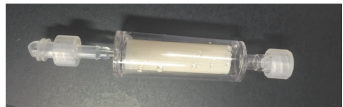
fig.3 Sterivex™-HV Sterile Vented Filter Unit with 0.45µm.
